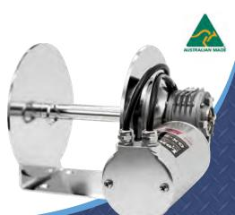
SPEC: 250MM DRUM 26MM SOLID SHAFT 88MM GEARSET 1000W MOTOR MAX DROP-RETRIEVAL SPEED: 46M/156 FT. P/M HOLDING AT ANCHOR: 3T ROPE/CHAIN CAPACITY: 90M X 8MM ROPE 7M X 8MM SL CHAIN RECC. BOAT SIZE: 5-8M PACKAGED WEIGHT (APPROX.): 22KG
