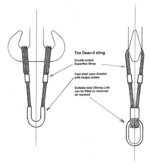
Dean-0 Slings are offered in seven different capacities with the WLL of: 11 tonnes, 20 tonnes, 40 tonnes, 60 tonnes, 80 tonnes, 110 tonnes, 165 tonnes. Suitable Master Links can be fitted into and removed from this sling as required. Dean-0 slings have been developed and are manufactured by:
