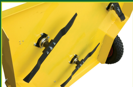
TRIPLE BLADE CUTTING SYSTEM
