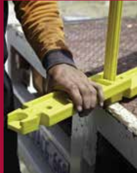
Assembling stile and rung
