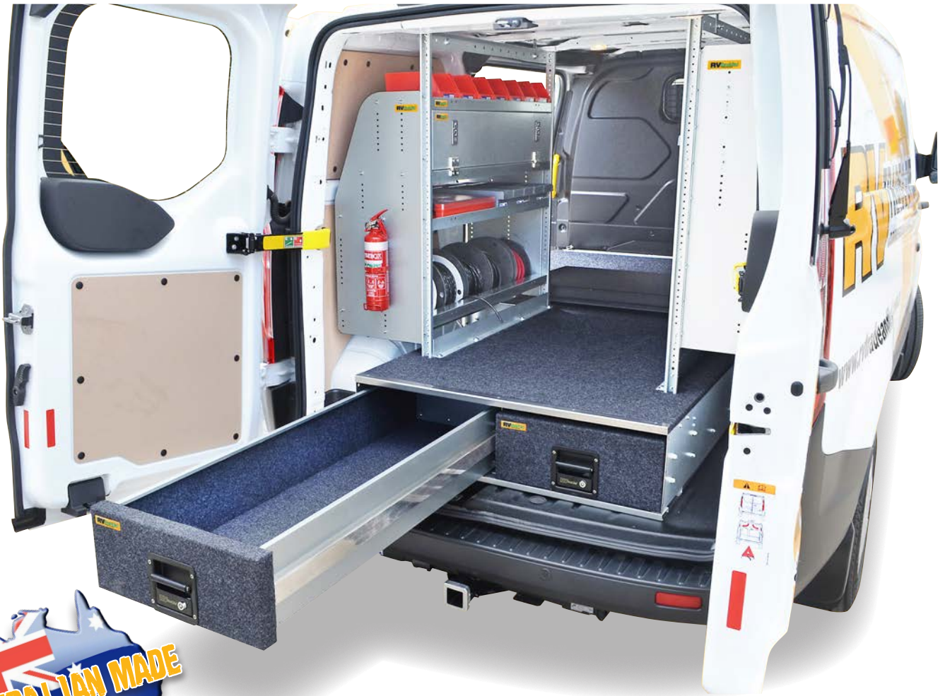
ABOVE: Ford Transit Van with Ecolite 1400 drawers and Ecolite van racks complete with plastic tubs and lockable security tool door. (Racks also available for Utes)
