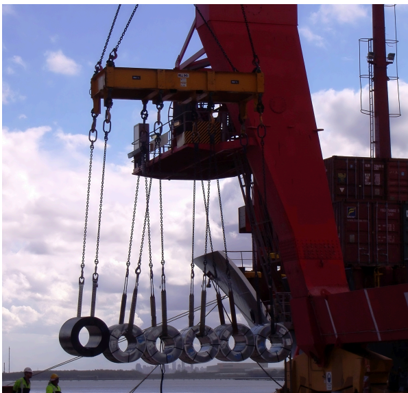
Type 1-A lifting steel coils off a freight ship.
