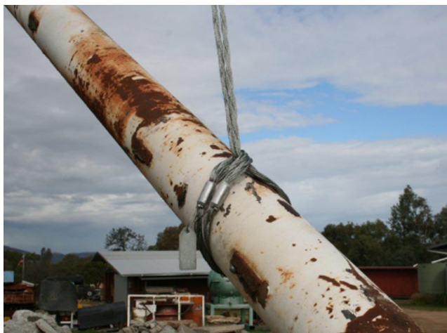
Steel pole lifted by a Superflex Strop as a choker
