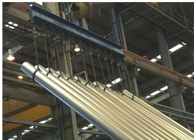
Multiple Stropps used as chokers in 'laydown' of hot aluminium billets.
