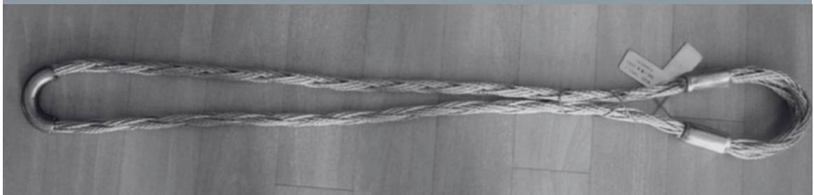
The same Strop untied from the knot. Note the minimal set remaining in the cable.
