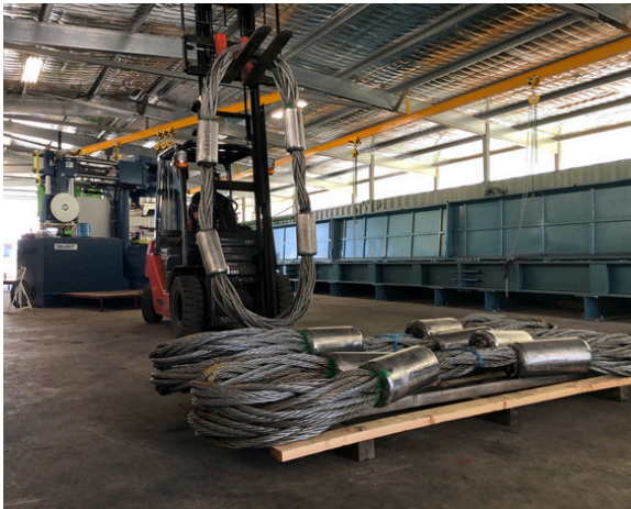
Our largest 24-0 cable as a Double Ended Strop held up by a forklift
