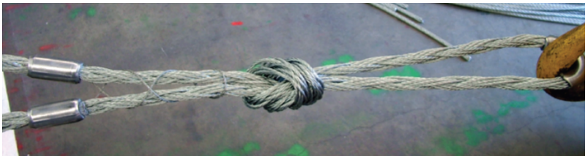
Superflex Strop, Size Three-5, with a hand tied knot under tensile load 400kgsf
