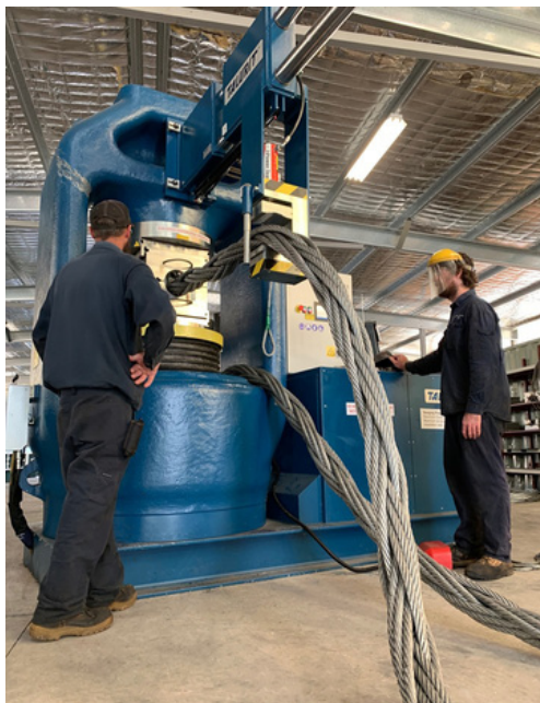
Our TwentyFour-0 Superflex Cable being pressed in our 4200 Tonne Talurit Swaging press.
