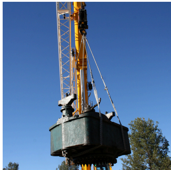
Type 1-C lifting the top of a swaging press.
