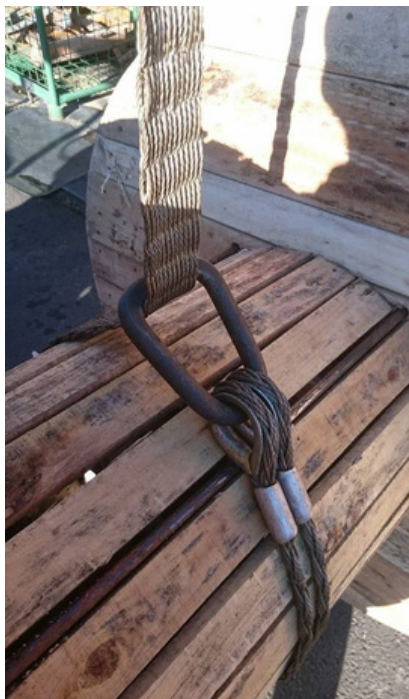
Type 2-R FWS displaying the choker usage on a timber reel
