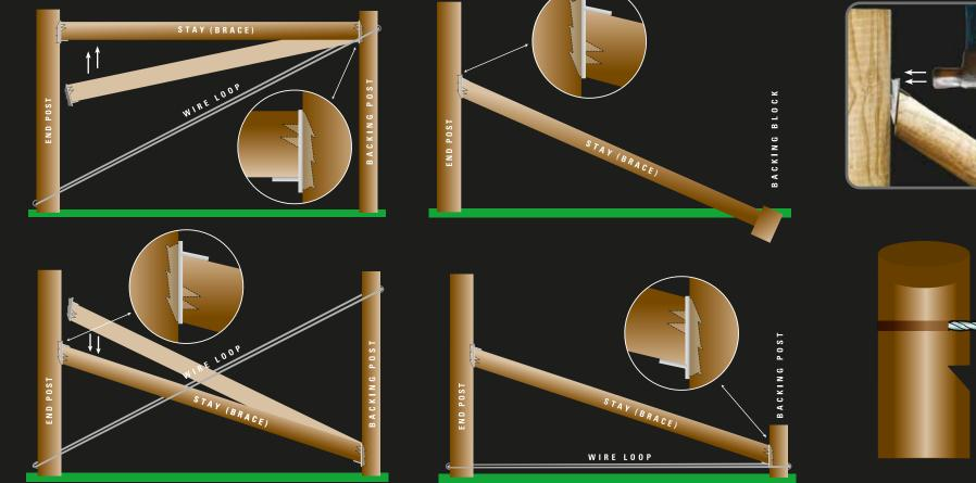
Cut the stay to suit the distance between both posts, allowing 5mm for the two brackets. Once the bracket is in position, a quick tap at the top of the bracket will lock it into position and stop it from riding back up the post
