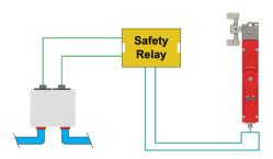
3. Upon reaching zero pressure, safety contacts change state to signal to safety relay.
