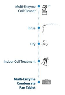
The **AerisGuard™** Multi-**Enzyme Condensate Pan Tablet** is an advanced multi-functional composition containing specifically selected enzymes & biocides to minimise biofilm formation in condensate drain pans and drain lines. Safe and effective removal and prevention of biofilm minimises the risk of blockages and condensate overflow. This minimises the risk of property damage.
