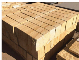
SPLIT SANDSTONE BLOCKS
