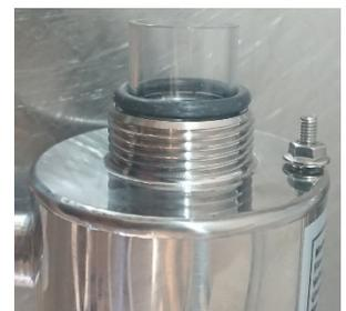
4. When the O-rings are seated, firstly loosely install the bottom nut and then the top nut until you feel resistance. Simultaneously tighten (by hand) the top and the bottom nut equally to keep the Quartz tube centred in the chamber. Do not apply any thread tape, grease, or sealant.
