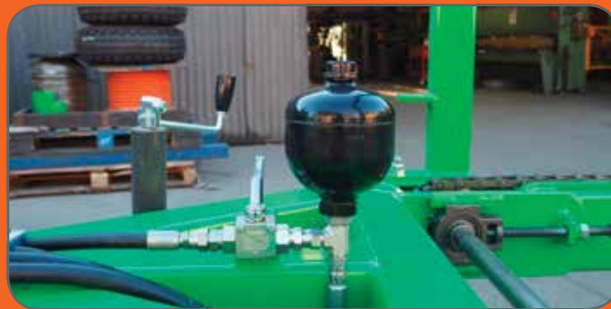
Soft ride hydraulic suspension accumulator
