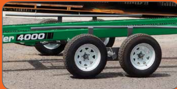
Walking beam dual wheel axle for a gentler ride over rough terrain
