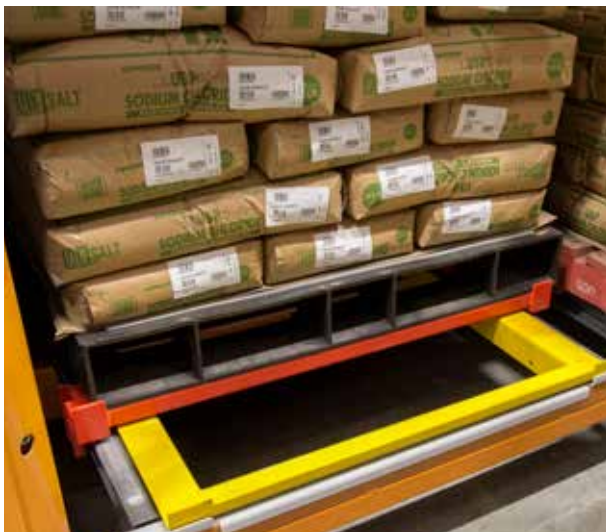
Push Back Pallet Racking Dense storage with greater selectivity
